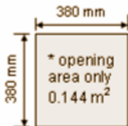
A. Does not conform to area requirements
